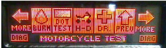
This will bring up the **HARLEY-DAVIDSON SPECIFIC MENU**. Similiar to "BEGIN PLAY TEST," this menu is used to test and adjust Game Specific Features. The feature in this game is **MOTORCYCLE TEST**. *Important*: The **Power Interlock Switch** must be pulled out for this Test to Function.
