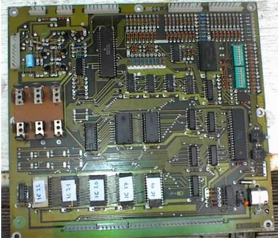
*Type 3 (with socket for IC14). I numbered the IC's so you can see what their place is. They do not have to be all present at the same time! Also notice of the orange dot at the bottom right, this is an added 33pF condo, why.. is explained further in this text.*
