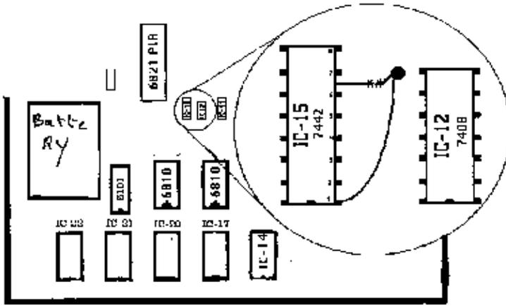
Find IC15, btween pin 6 and 7 there's a trace which goes to a round solder point. Cut this trace and connect the round solder point with pin 1 of IC 15. That's it !!!!!!!
