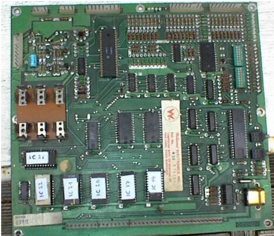
*Type 4, you see an extra ic socket for IC26. Here also the ic's are numbered for clarity, but not all of these IC's must or may be present at once on the board.....*
