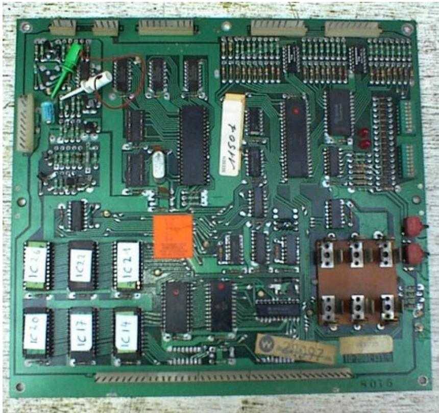
*A type 6 board with the battery-holder on the right, i numbered the ic's so you can see where there emplacement is. Not all of them are always present on the board!! Remarque the jumper in the left top corner, he connects resistor R27 and condensor C23 ( both upper sides)and is neccessairy to work on the test-fixture when only the 5 volt is connected as explained under 'manual '.*
