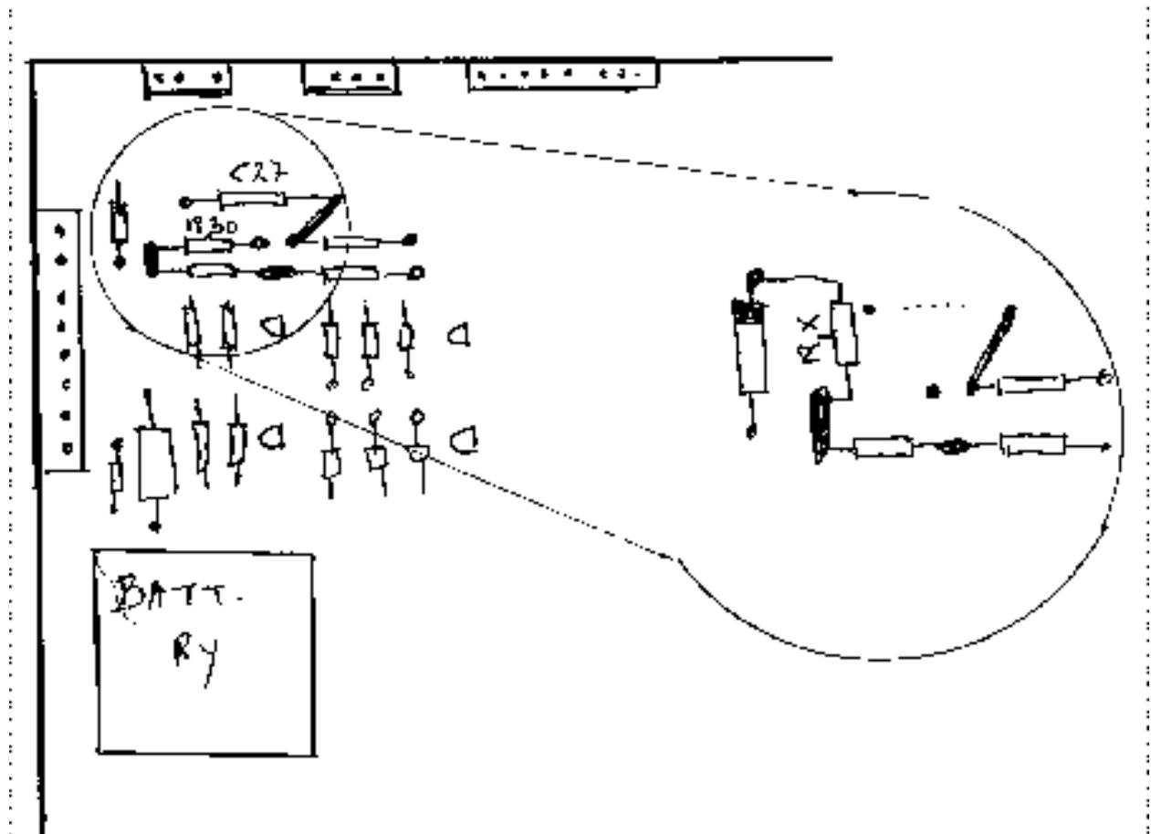
Search in the top left corner 5 transistors and several resistors. There are 4 horizontal resistors with just above them a condenser. It's ok to remove this condenser (c27), also resistance top left (R30). Add a new resistor (Rx) of 10K–ohm like shown in the drawing, between the top side of the zener–diode and the left connecting point of the removed R30. That's it...
