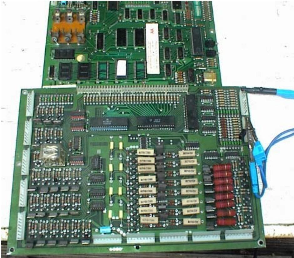
*Here's the setup to test the driver board. Connected to the cpu, in IC17 is my test-eprom, and you'll notice both sockets next to it have been replaced..*
